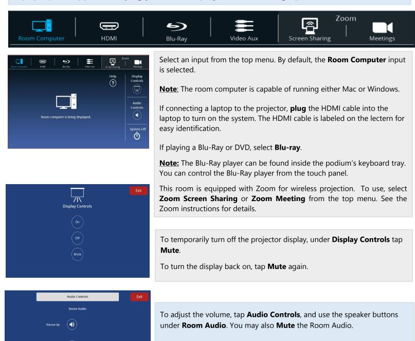
To turn off the projection system, tap **System Off**. A pop-up will appear asking you to confirm shutdown. A pop-up then appears notifying you that the projector is cooling down.
