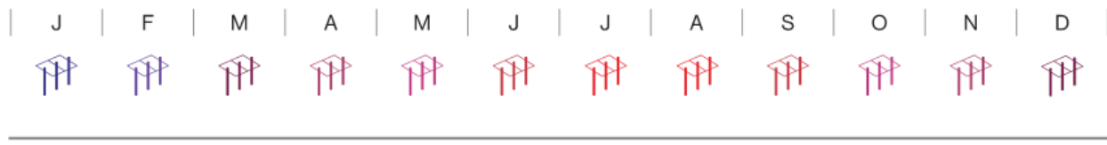
Figure 7: Artist depiction of annual operation of a ground source heat exchanger cooling down in winter months as heat is extracted from the ground and warming up during the summer as heat is rejected from buildings to the ground.
