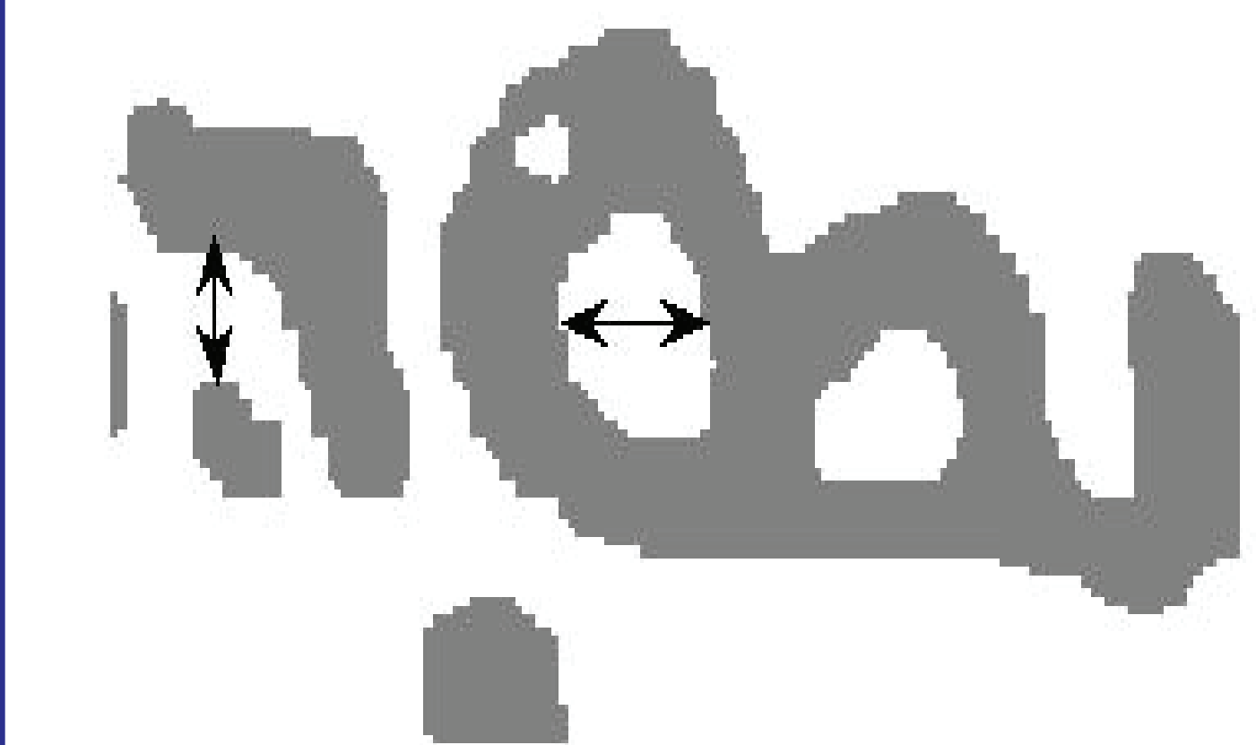
Figure 4: Schematic showing examples of run-lengths on background both vertical and horizontal.
