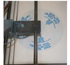
Print head binding powder in layer of SolidWorks design.
