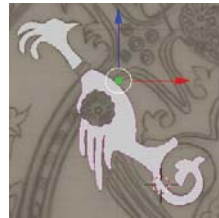
One phoenix, modeled in 2D by Bezier curves, and extruded into 3D.
