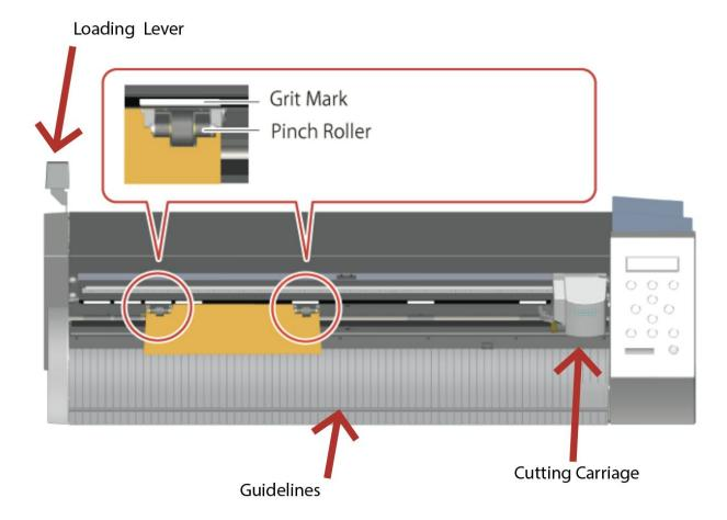
Unspool a bit of material at the back of the machine, you don't want the roll to be tight.
